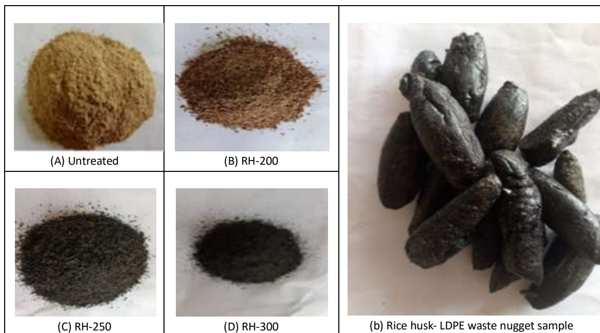
Fig. 2(a) Images of rice husk (A, B, C and D) and (b) rice husk- LDPE waste nugget sample
