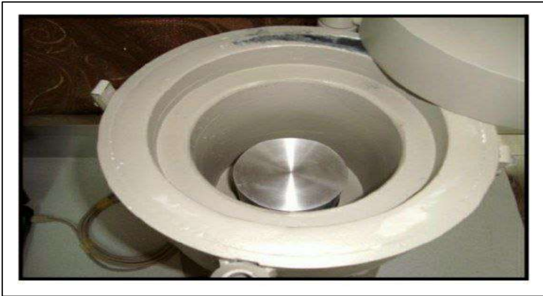
Fig. 4. Image of the detector inside the shielding chamber[12].
