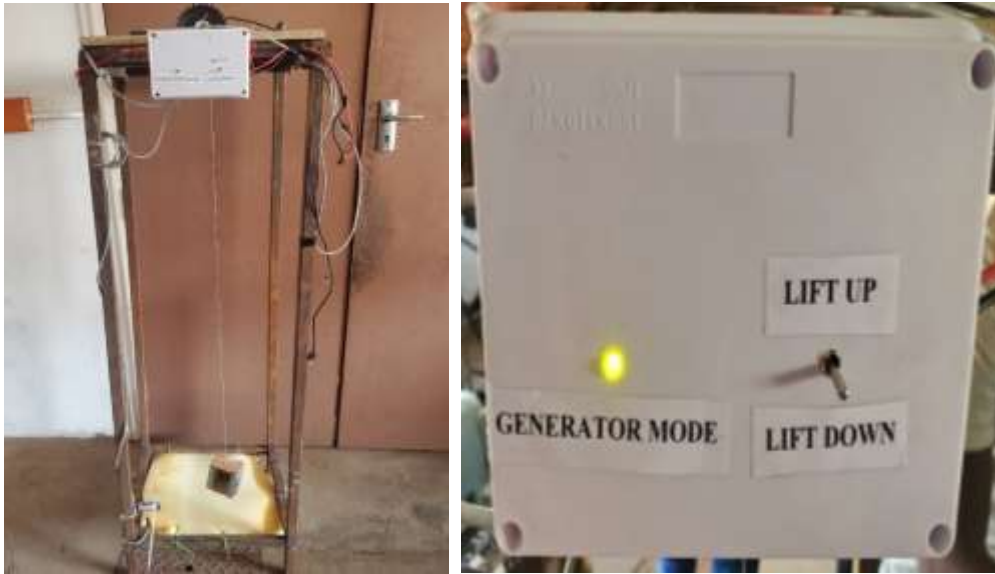
Figure 3: The designed prototype modelling a vertical lift system Control box indicating that the system is in generator mode
