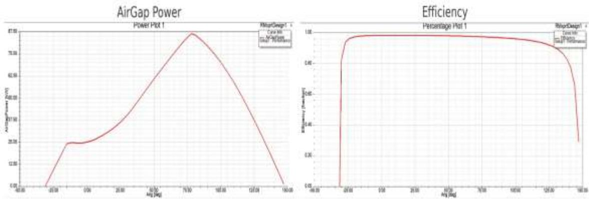
Figure 12 RMxpvt Results for Air Gap 3.5
