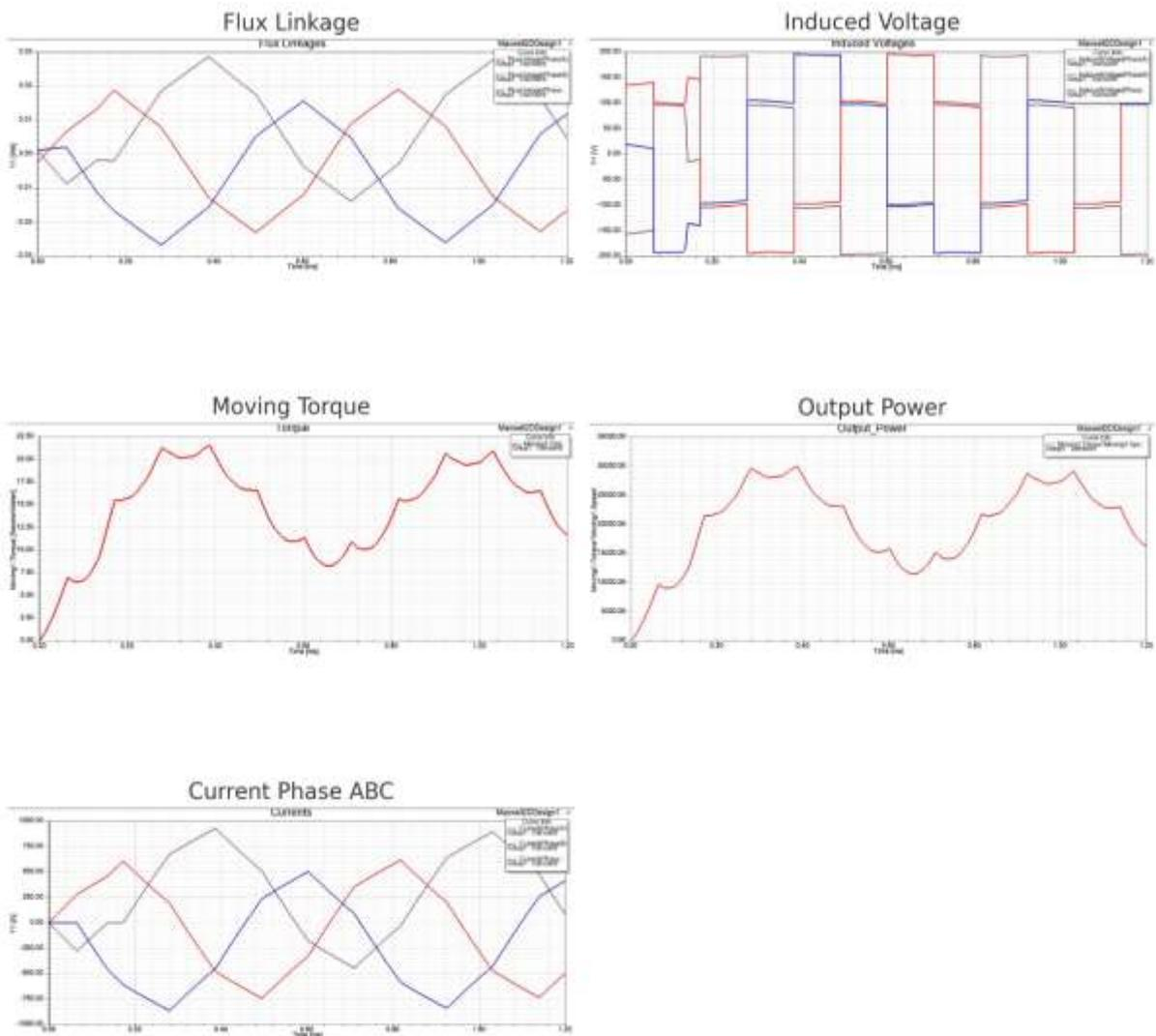
Figure 2 Maxwell 3D Results for Cobalt
