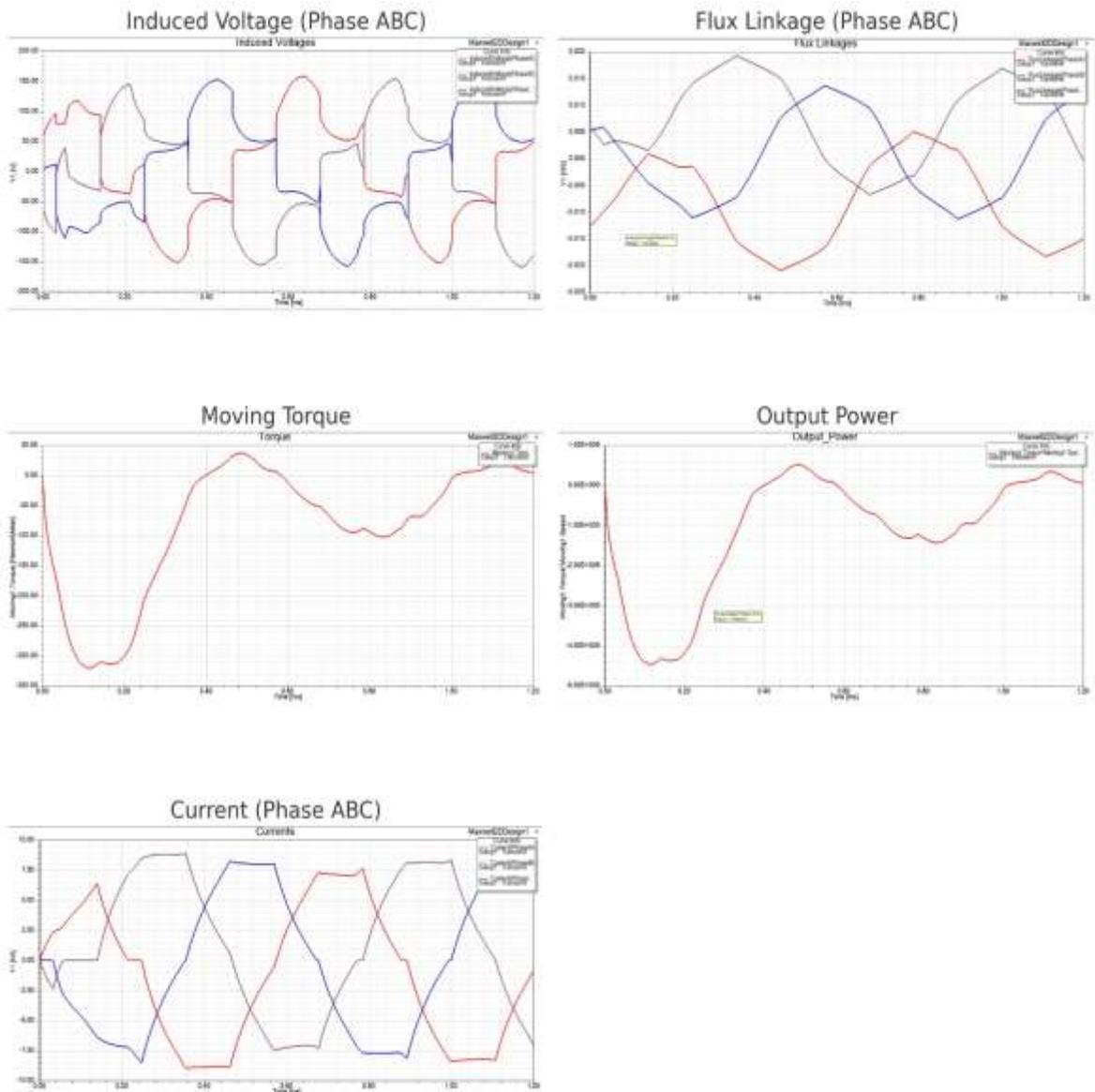
Figure 16 Maxwell 2D Results for Air Gap 4.5
