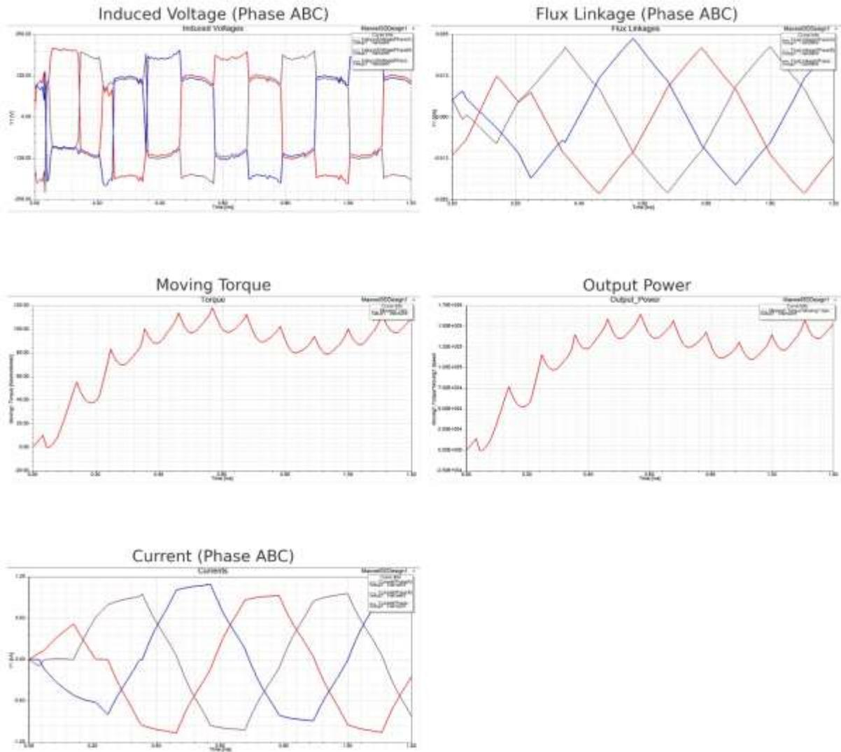
Figure 17 Maxwell 3D Results for Air Gap 4.5
