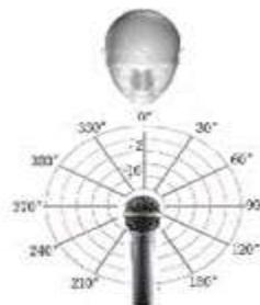
Figure 1 Method to determine the sensibility pattern of a microphone.
