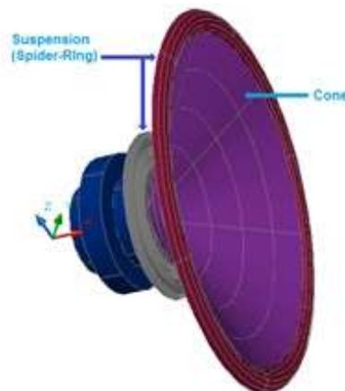
Figure 6 Low frequency loudspeaker parts.
