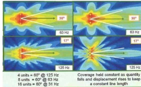
Figure 14 Spacing effects – “steering” a coupled line source arrays of loudspeakers [10].
