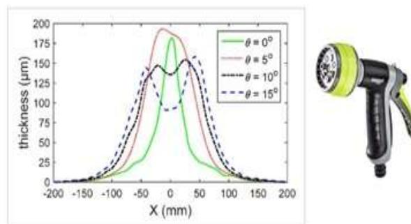
Figure 16 Coating thickness profiles along the x-axis for different  $\theta$  values when  $L = 30$  mm [11].
