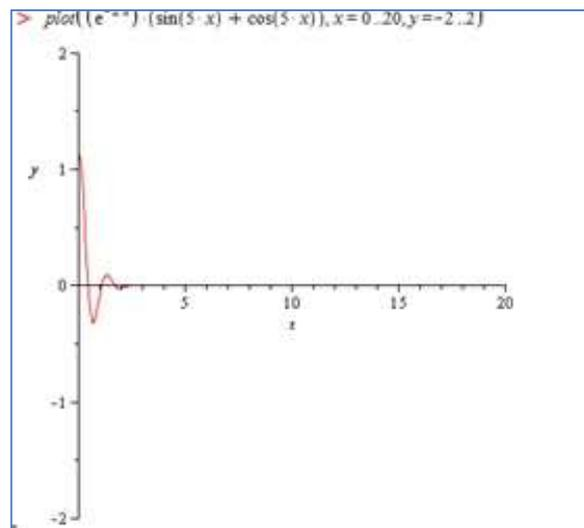
Figure 7 Plot for function  $y = e^{-2x}(\sin(5x) + \cos(5x))$
