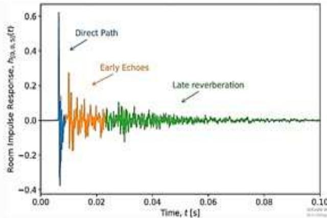
Figure 5 Measure of reverberation time in a closed-model room.
