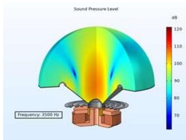
Figure 10 A 3D Loudspeaker frequency spectrum at 3500Hz [8].
