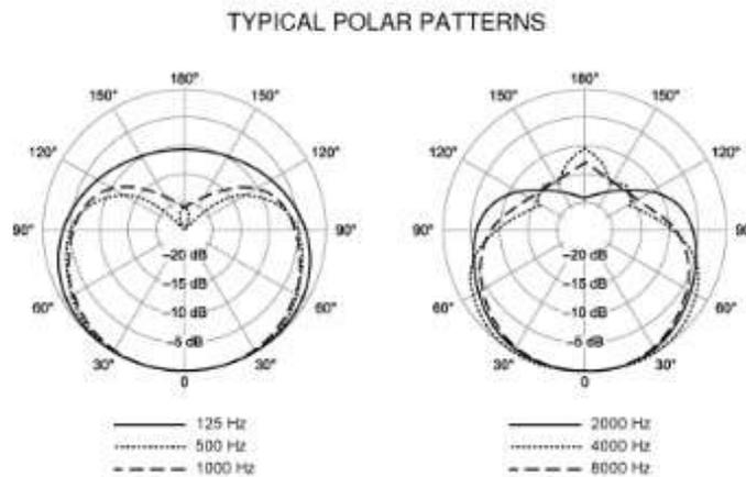
Figure 3 Polar pattern of a Shure™ SM-57 Microphone
