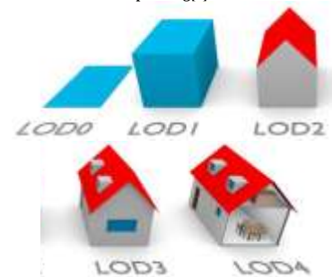
Figure (3): Biljecki's division of modeling according to Level of Detail [11]
