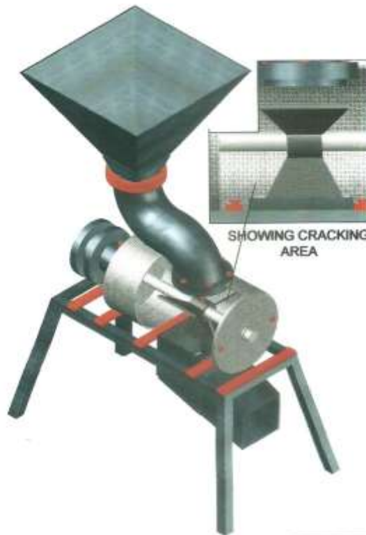
Fig. 1: Pictorial view of an S-neck palm nut cracker
