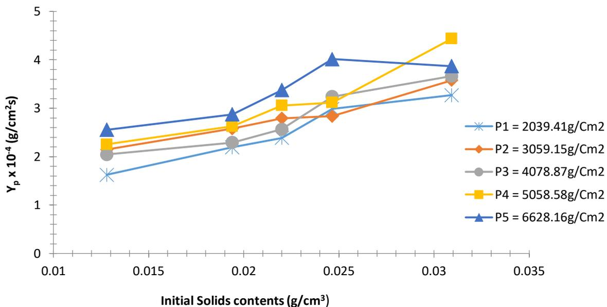
**Figure 5: Variation of Yield (Y<sub>p</sub>) with Initial Solids content for 17.81% Conditioned sludge at various Pressures.**
