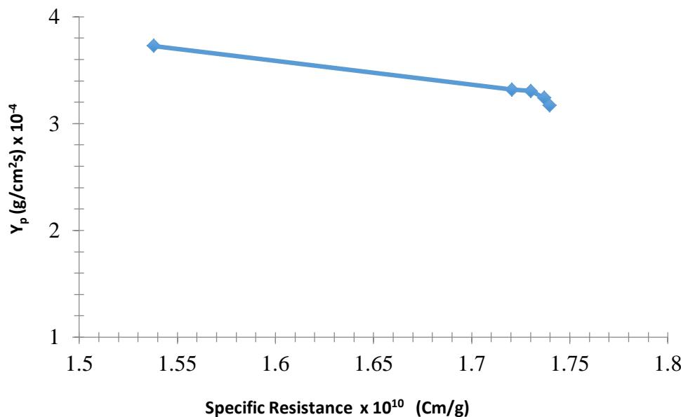
**Figure 6: Effects of Specific resistance on Cake yield at a pressure of 4078.87 g/cm<sup>2</sup>.**
