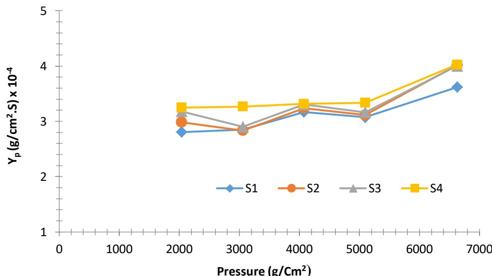
**Figure 3: Effects of Operating Pressures on Filter Yield**
