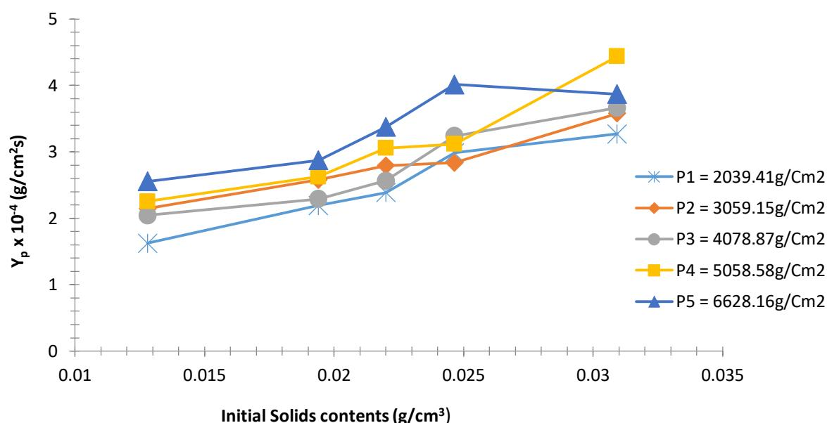
**Figure 5: Variation of Yield ( $Y_p$ ) with Initial Solids content for 17.81% Conditioned sludge at various Pressures.**
