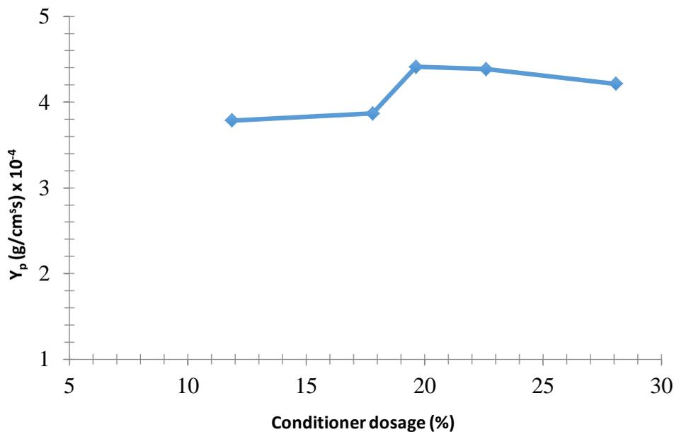
Figure 4: Effects of Conditioner dosages on Cake yield at a Pressure of 5098.58  $\text{g/cm}^2$
