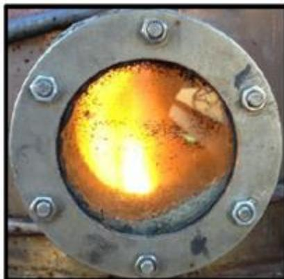
Fig. 6: Photograph of the flames from the combustion of pomace olive.
