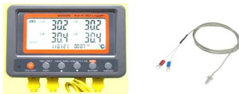
Fig. 4: Photograph of k-type thermocouple with digital display
