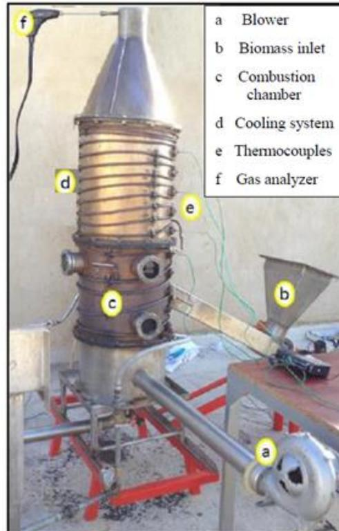
Fig. 3: Photograph of the biomass boiler in operating mode.
