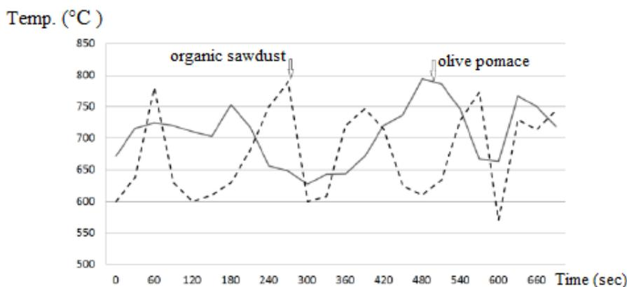
Fig.7: Evolution of the temperature of gases from the burning of pomace and sawdust in within the boiler
